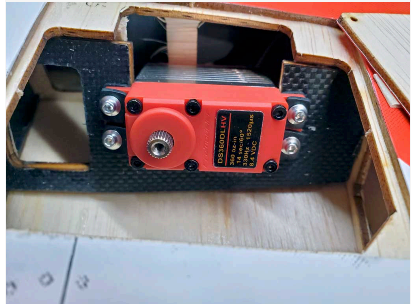
Internal side mounted servo can be tricky to reach with tools and especially securing bolts
