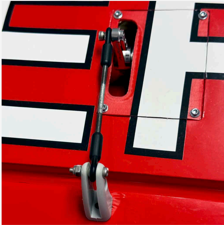
The hatch mounted servo with PDRS32-25T servo horn uses a ball link equipped pushrod
