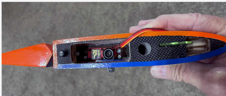
Total pain in the ass side mount servo install is accessed through the root rib after removing the stab
