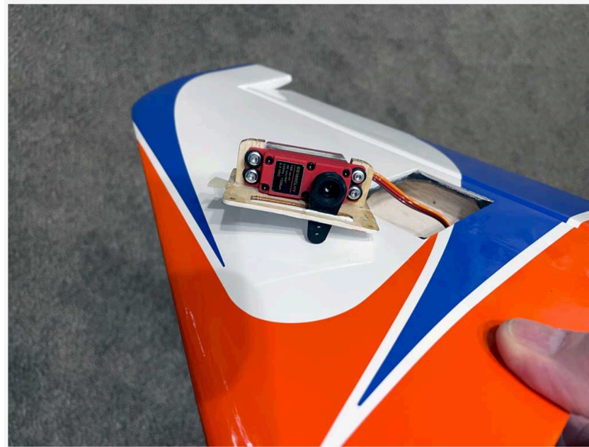
It doesn't come more simple than a plate mount installation – suitable for ailerons, flaps, and stabs
